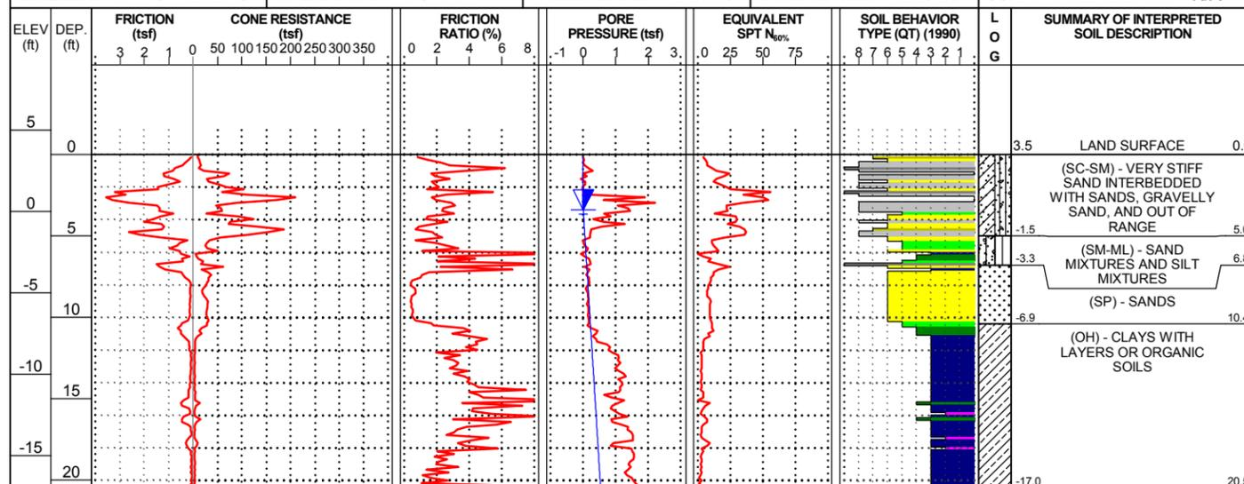
Boring Terminated at Elevation -17.0 ft
