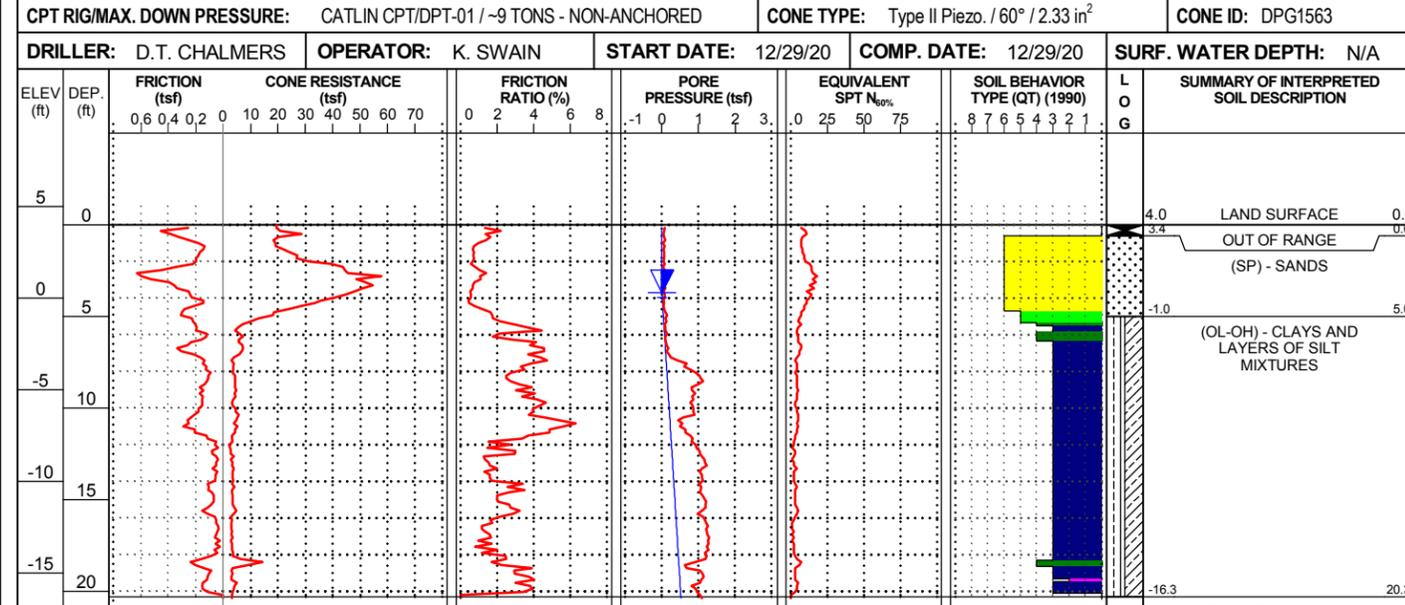
Boring Terminated at Elevation -16.3 ft
